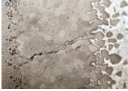
Figure 7. Aluminium canals formed during dipping of niobium in molten aluminium.
