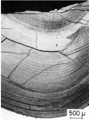
Figure 10. Regular laminated oxide in a heavy corroded boiler tube.
