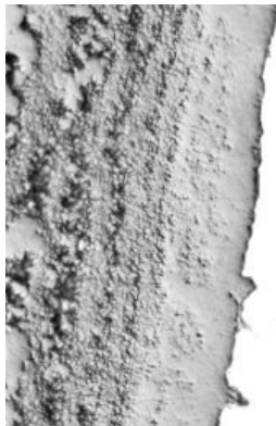
Figure 14. Corroded boiler tube. The numbers of pores increase at longer distances of the oxide-metal interface.
