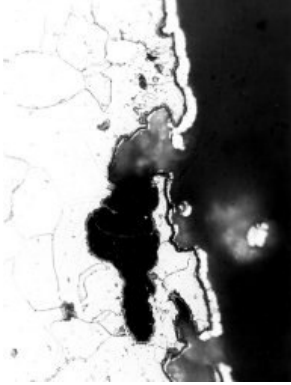
Figure 13. Dehydrated rust-layers on concave places of the rough boiler tubes. The rust has been formed during the many shutdowns.
