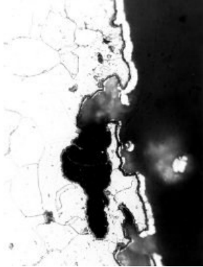
Figure 13. Dehydrated rust-layers on concave places of the rough boiler tubes. The rust has been formed during the many shutdowns.
