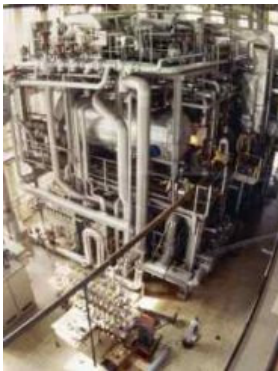
Figure 1. Experimental 1 Mw boiler for corrosion experiments at KEMA (the Netherlands).
