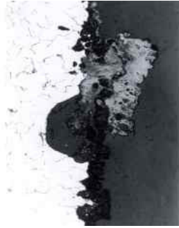
Figure 11. Pimple shape deposits, formed under plug-flow and bubble-boiling conditions.
