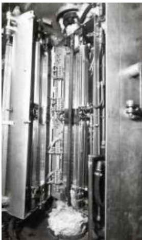
Figure 3. Test tube for heat-input measurements with opened furnace in test section II.
