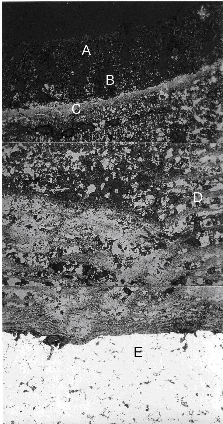
Figure 4: Characteristic oxide scale on corroded boiler tubes. The 4 stages of the corrosion process can be recognized in the oxide crust. A: Porous layer of oxide deposits, B: Salt layer, C: Top-layer, D: Laminated oxide, E: Steel.
