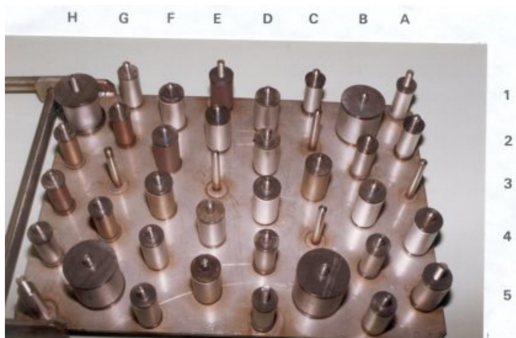
Figure 3 Samples mounted in the rack, before exposure. Flow direction from left to right.
