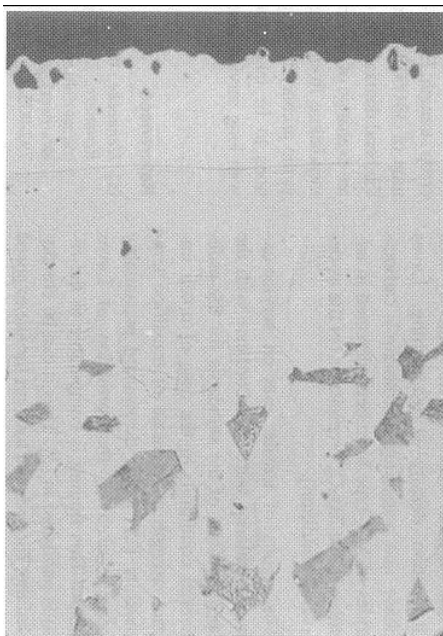
Fig. 1b. Cross-section (light microscope) through a Cr diffusion coating on 10CrMo910 (etched with Nital). The coating is located at the top, with a decarburized zone underneath and at the bottom the normal steel structure of ferrite with perlite islands in it.
