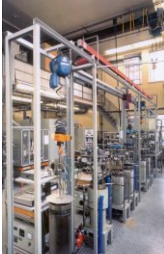
Figure 1. The water conditioning system and autoclaves for SSR and LCF testing
