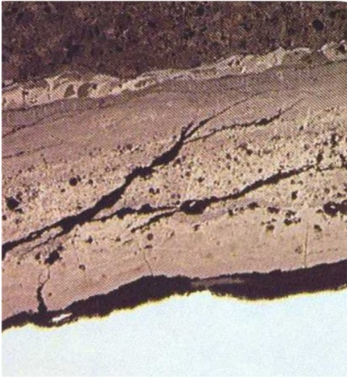
Figure 1. Optical microscopic image of the fire side tube deposit.
