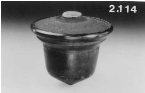
Spindle under high flow condition. Top was not coated. (photo KEMA). (2.114)
